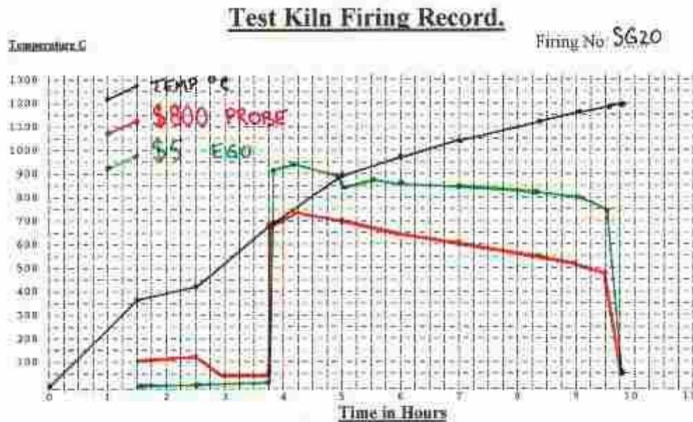
Reduction was commenced in this firing at about 700 degrees C, by closing the damper just enough. You'll notice how both red and green lines on the graph shot up together abruptly as
