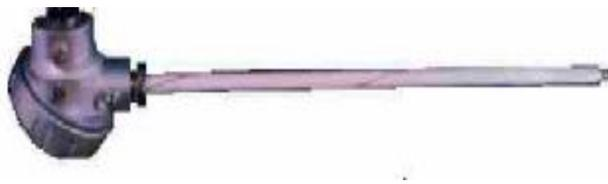
In a kiln oxy-probe, the little zirconium oxide pellet is fixed to the end of a long hollow alumina tube, so it can be poked down through the thick kiln wall into the hot interior.
