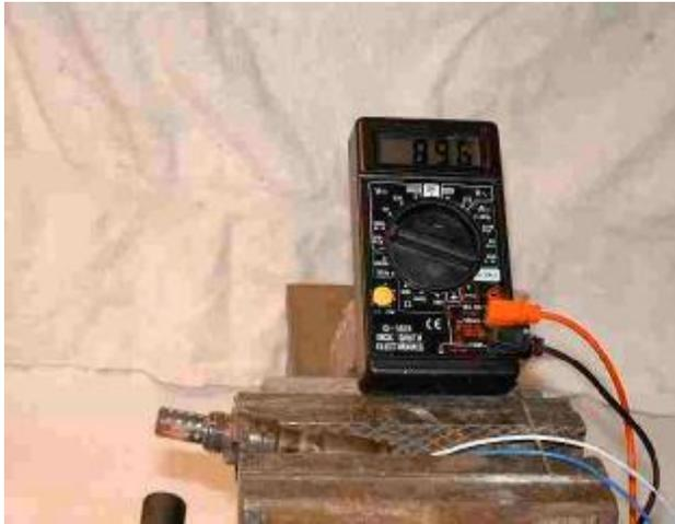
Clamp the sensor in a vice, or use multi-grips. Clip the meter onto the leads (this is easiest with a 2-lead sensor. If there's only one lead, then the body of the sensor is the other side of the signal). Play the flame from the gas torch onto the perforated metal thimble of the sensor, and expect an instant rise in the meter reading. You can heat the thimble red hot with no risk of damage. An output signal of 700 or 800 millivolts is not unusual, but only if the gas flame is starved for oxygen.
