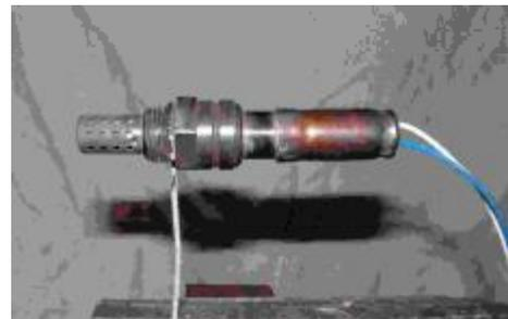
In both cases, one side of the pellet is exposed to the hot gases, and the other side is in contact with clean ordinary air. The voltage given out by the probe tells us what we want to know about the oxygen concentration in the hot gas.
