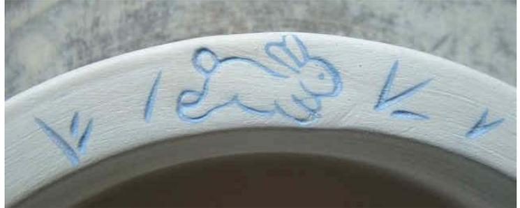
You're unlikely to find little gaps in the imprints after the bisque firing, but if you do it's possible to make minor alterations even at this late stage. With a sharp tool you can scrape out a groove if it's really necessary, and dab in a little more slip. For just a small repair, it's OK to raw-glaze over the top of the repair, and you'll never notice.
