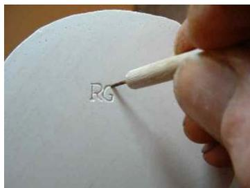
When the plaster sets hard, the pancake should lift off easily. Engrave the pattern you want into the flat surface with a pointed tool such as the end of a big safety pin. Aim for deep narrow grooves rather than broad flat shallow ones. For your initials, the letters don't have to be reversed. Do them the right way round. There's no need to wait for the plaster to become completely dry. It engraves more easily if you do it sooner.
