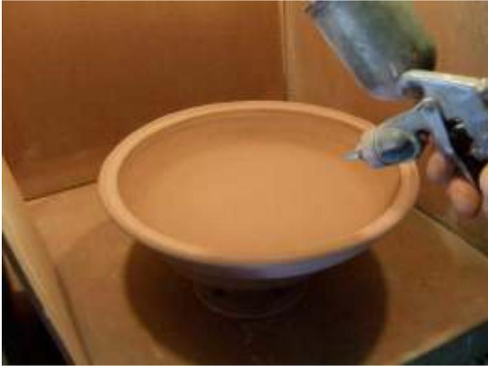
Now let's look at how the glazes are applied. In this picture, the underside of a platter rim has already been sprayed. The platter has been turned over, right side up, and a measured quantity of chocolate glaze is being sprayed evenly on the top.
