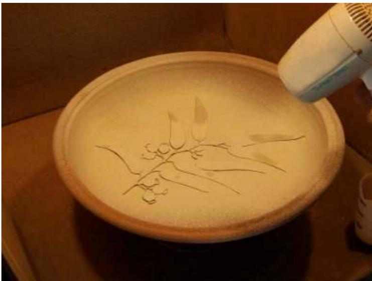
If a pool of wet glaze builds up on the stencil, stop spraying and blow gently with warm air until it's dry before continuing.
